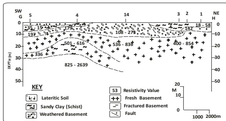
Fig. 10: B) Geoelectric Section and Probable Geological Interpretation Along Profile G – H.
