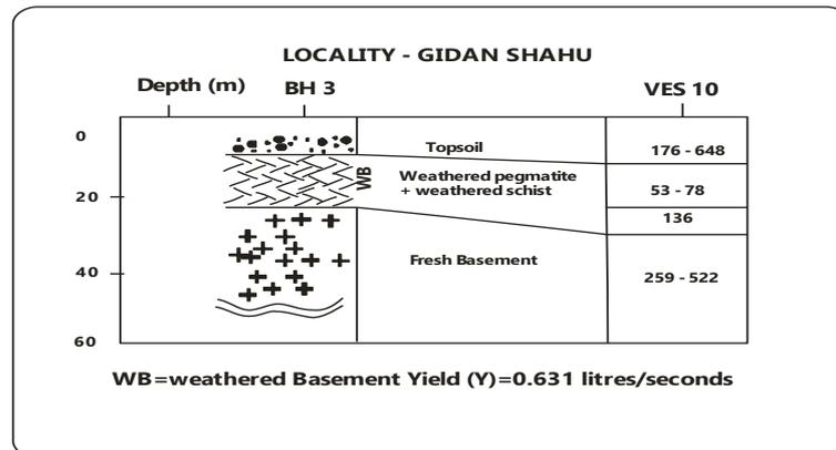
Fig. 12: Comparison of the Interpreted Geoelectrical Section (VES 10) and the Borehole Lithological Section.
