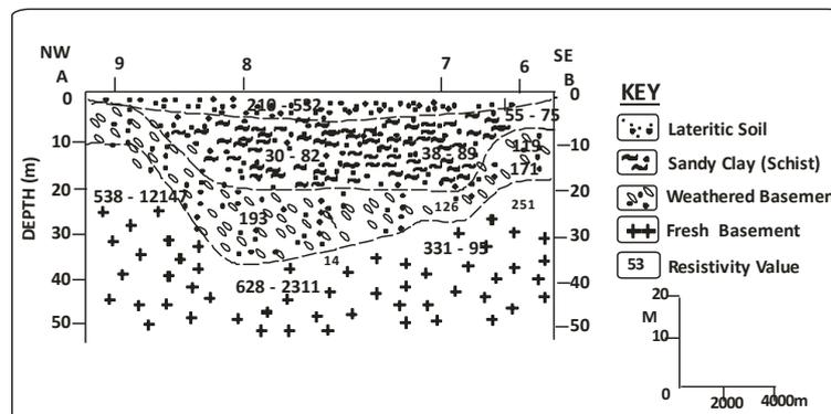
Fig. 7: B) Geoelectric Section and Probable Geological Interpretation Along Profile A – B.
