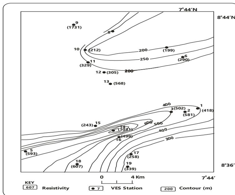
Fig. 4: Map of Apparent Resistivity for AB/2=95m.
