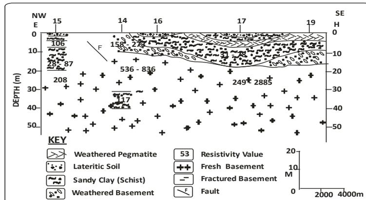
Fig. 9: B) Geoelectric Section and Probable Geological Interpretation Along Profile E – F.
