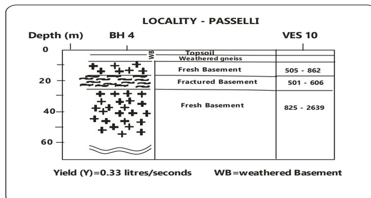
Fig. 14: Comparison of the Interpreted Geoelectrical Section (VES 4) and the Borehole Lithological Section.
