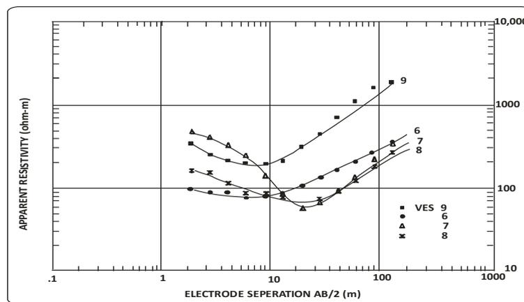
Fig. 7: A) VES Sounding Curves Along Traverse A – B.
