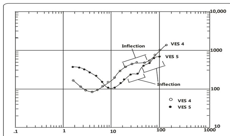
Fig. 6: Depth Sounding Field Curve (Fractured Layers) of the Study Area.
