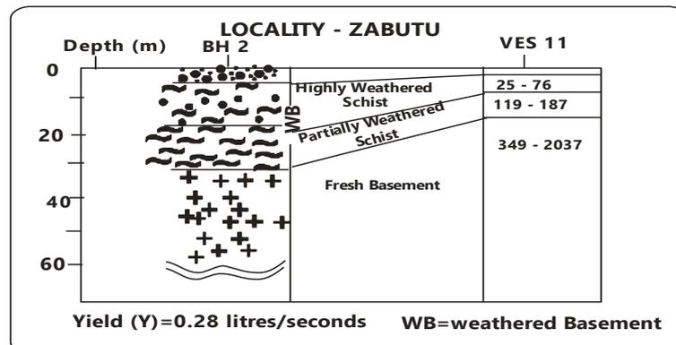
Fig. 13: Comparison of the Interpreted Geoelectrical Section (VES 11) and the Borehole Lithological Section.
