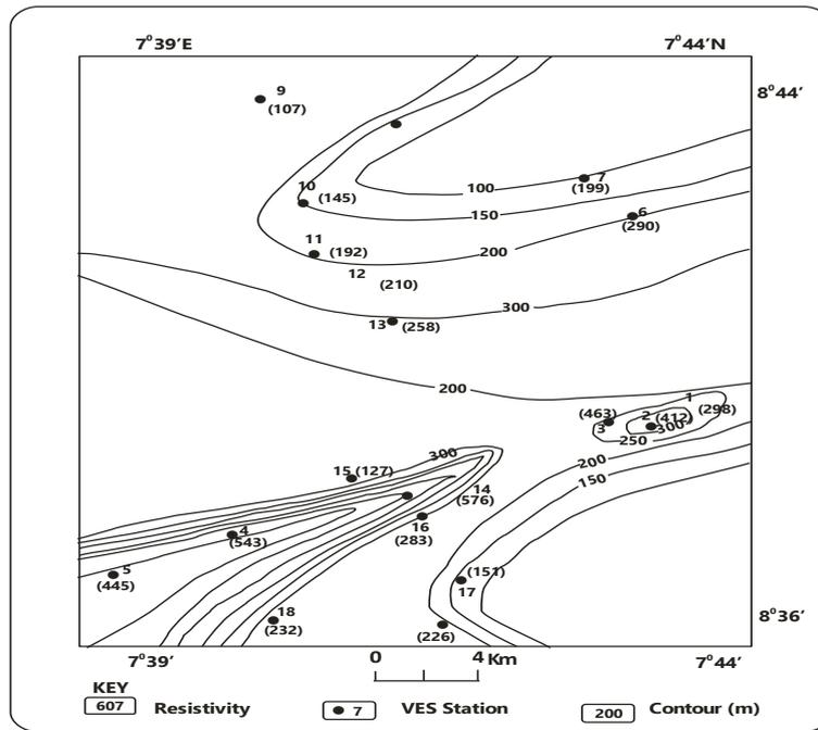
Fig. 3: Map of Apparent Resistivity for AB/2=55m.
