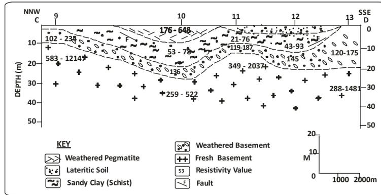
Fig. 8: B) Geoelectric Section and Probable Geological Interpretation Along Profile C – D.
