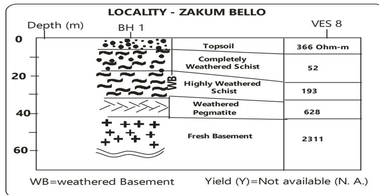
Fig. 11: Comparison of the Interpreted Geoelectrical Section (VES 8) and the Borehole Lithological Section
