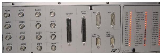
Fig. 2: dSPACE Connector Board.
