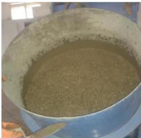
Fig. 2: Fresh Geopolymer Concrete.
