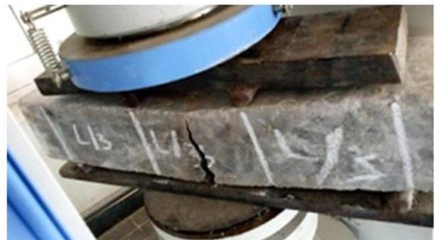
**Fig. 3:** Showing Prism Testing.
