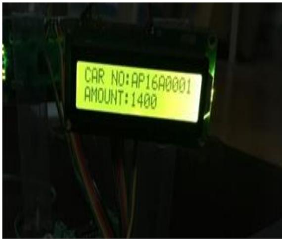
Fig. 9: Car Number and Account Balance Display.
