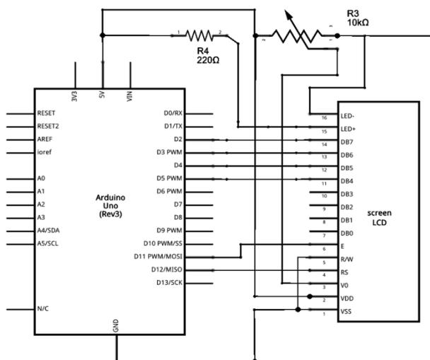
Fig. 6: LCD and Aurdino Interfacing.
