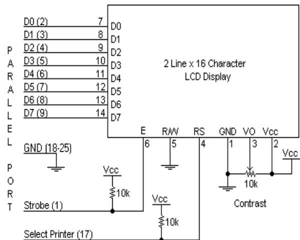
Fig. 5: Pin Diagram of LCD.
