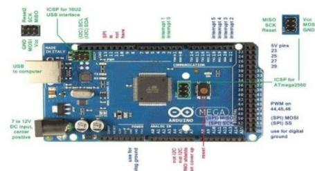
Fig. 6: Arduino Mega 2560 Pins Configuration.
