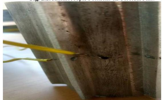
Fig. 2.2: Thermocouple Attachment on Splines of Fins.
