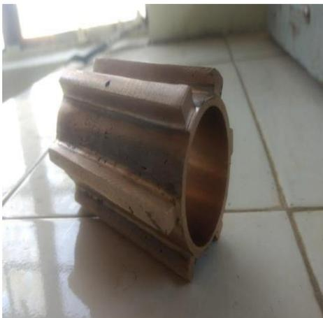
Fig. 2.6: Gun Metal Toroidal Fin.
