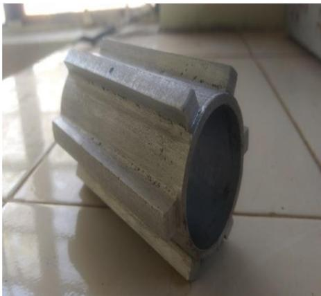
Fig. 2.5: Aluminium Toroidal Fin.
