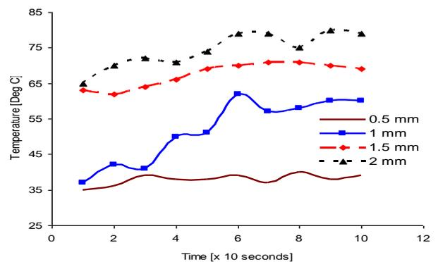
Fig. 6: Temperature Variations for HSS Tool Cutting Aluminum at 625 Rev/Min.
