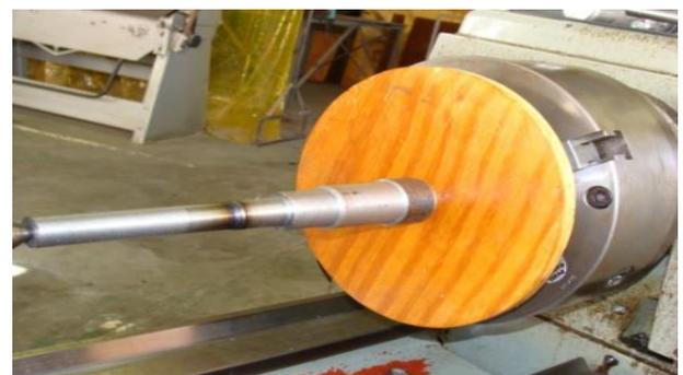
Fig. 12: Prevention of Air Flow from Chuck Jaws.
