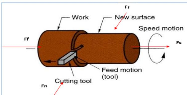
Fig. 2: Forces Acting on A Tool.
