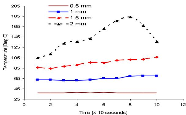
Fig. 8: Temperature Variations for Tungsten Carbide Tool Cutting Mild Steel at 625 Rev/Min.
