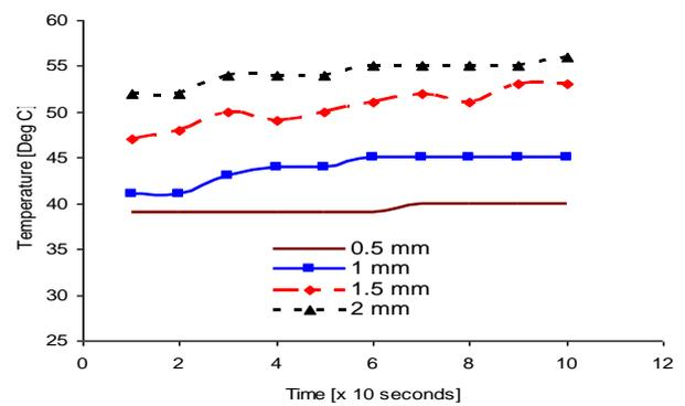
Fig. 4: Temperature Variations for Tungsten Carbide Tool Cutting Aluminum at 625 Rev/Min.
