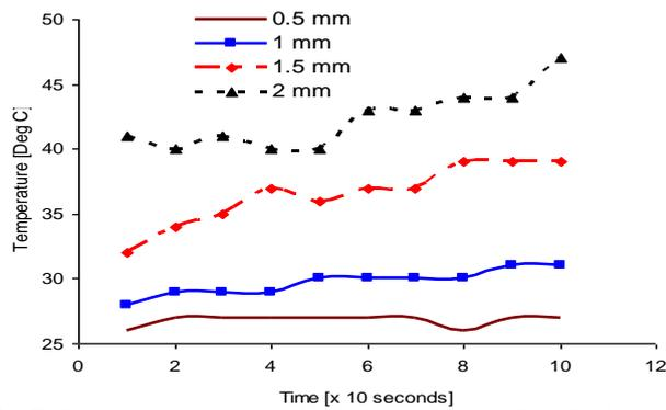
Fig. 7: Temperature Variations for Tungsten Carbide Tool Cutting Mild Steel at 470 Rev/Min.
