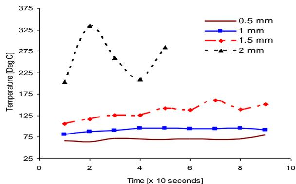
Fig. 9: Temperature Variations for HSS Tool Cutting Mild Steel at 470 Rev/Min.
