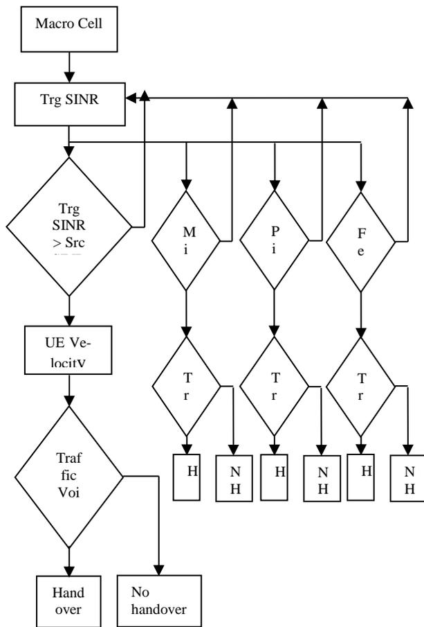
Fig. 4: Selecting A Particular Cell and Performing Handover.
