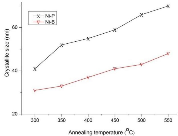
Fig. 6: Comparison of Crystallite Sizes of Ni-P and Ni-B Coatings.
