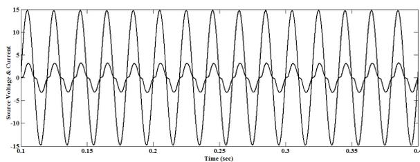
**Fig. 8:** Line Current (A) & Voltage (V) At 230V, 50Hz Supply.
