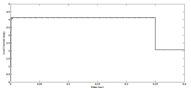
**Fig. 14:** Load DC Current with Change of Load.
