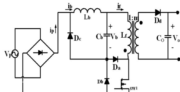
Fig. 1: Integrated PFC Converter.
