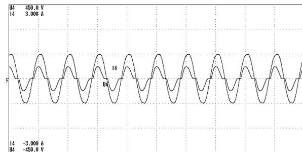
Fig. 17: Experimental Results for Source Voltage (V) and Current (A) for 110V (RMS) at Full Load.
