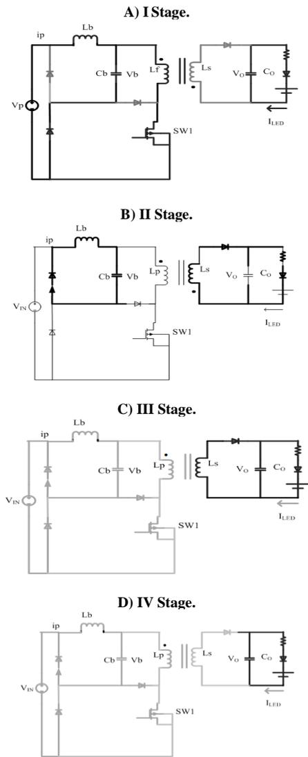
Fig. 2: Operating stages of Integrated PFC Converter.
