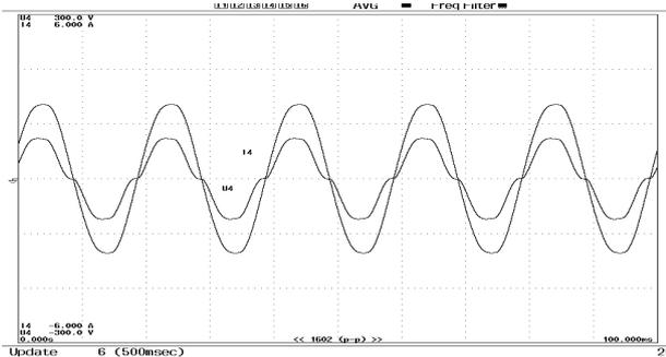
Fig. 16: Experimental Results for Source Voltage (V) and Current (A) for 230V (RMS) at Full Load.
