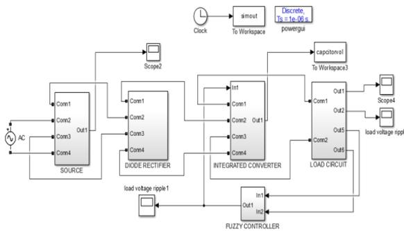
**Fig. 7:** Matlab/Simulink Model of Fuzzy Peak Current Controlled Integrated PFC Converter.
