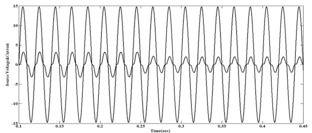
**Fig. 12:** AC Source Voltage & Current Step-Change at 0.25sec.
