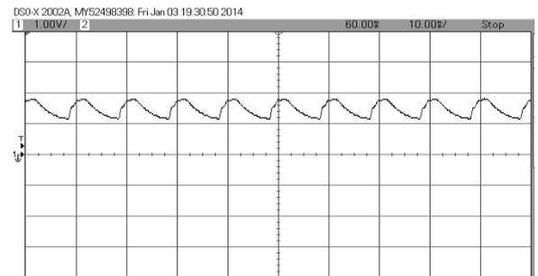
Fig. 19: Bulk Capacitor Voltage.
