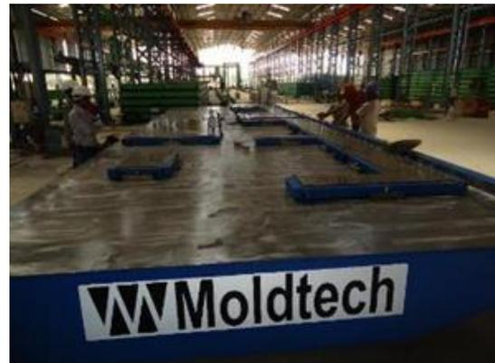
Fig. 6 Wall/ Slab casting tables
