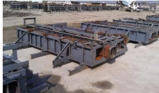
Fig. 5 Shell Column Mould
