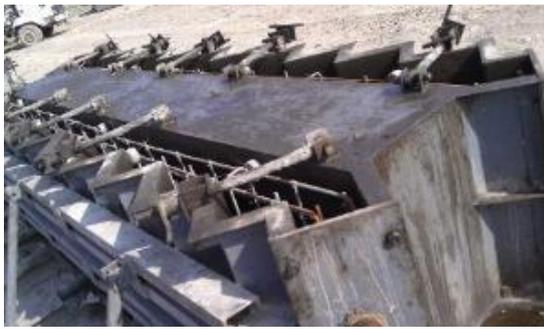
Fig. 8 Pre-cast Stair case mould
