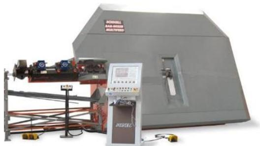
Fig. 10 Automatic dual-direction stirrup bender
