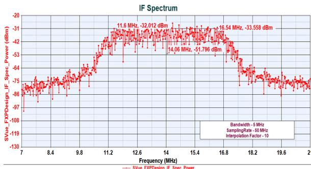
Fig. 9: IF Output Spectrum.
