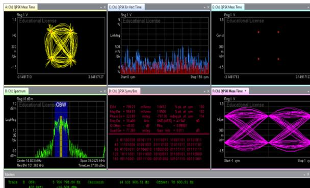
Fig. 25: VSA Output for FPGA Implemented IF Section.
