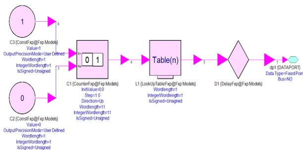
Fig. 2:Schematic Representation of PN Generator.
