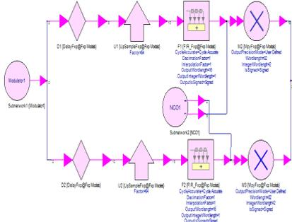
Fig. 14: Schematic Representation of RF Section.
