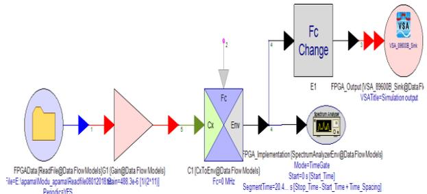
Fig. 23:Schematic Representation of IF Section with FPGA Output Data as Input.
