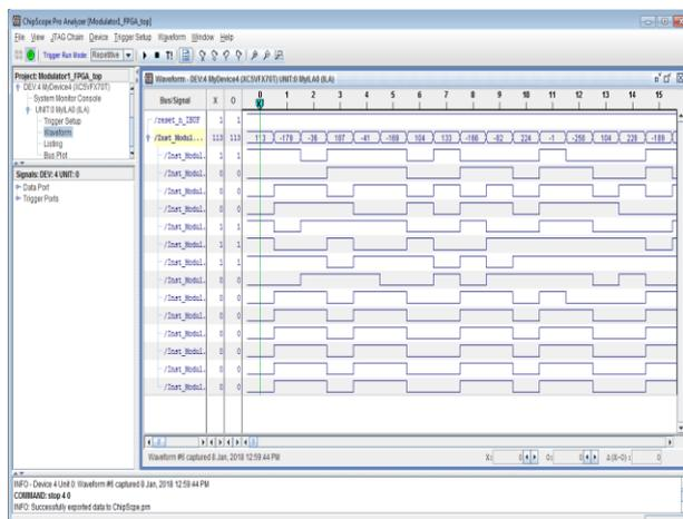
Fig. 22:Output of ChipScope Pro Analyzer.
