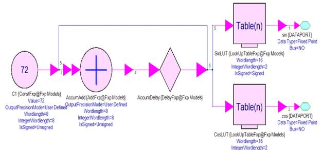
Fig. 11: Schematic Representation of NCO1.
