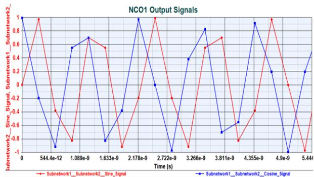
Fig. 12: Sine and Cosine Output Signals of NCO1.
