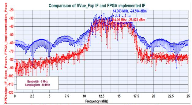
Fig. 24:Comparison of Systemvueand FPGA Implemented IF Section.
