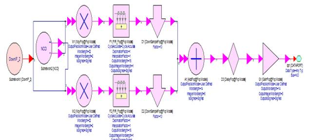
Fig. 19: Schematic Representation of Downconverted Baseband Section.
