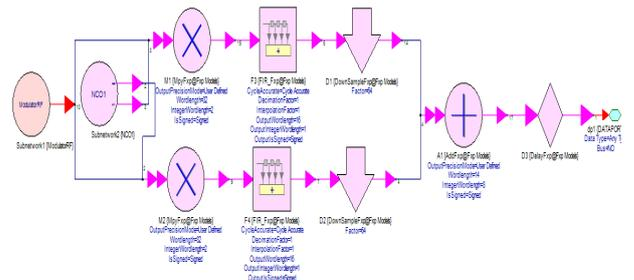
Fig. 17: Schematic Representation of Downconverted IF Section.
