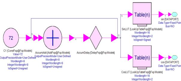
Fig. 6: Schematic Representation of NCO.
