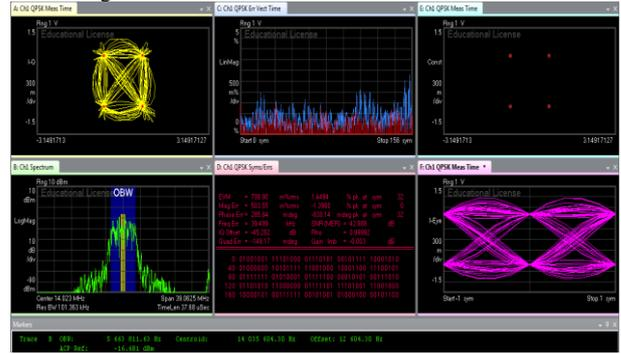
Fig. 10: VSA Output at IF Section.
