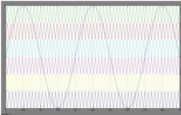
Fig. 6: POD PWM for 7-level MLI
