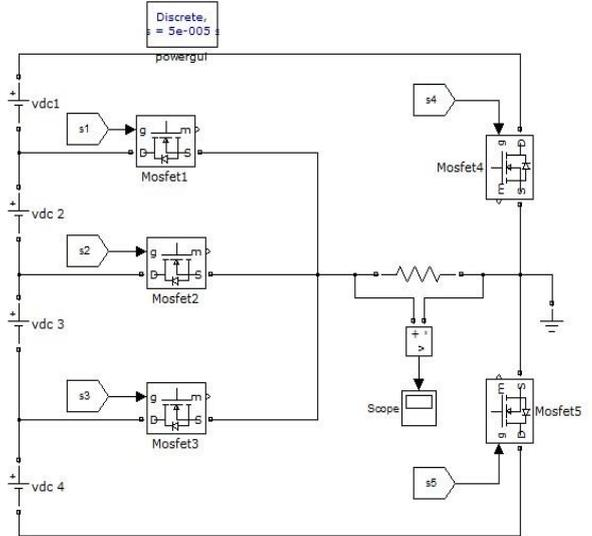
Fig. 2: Simulation circuit for 5-Switch 7-Level Topology
