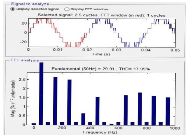
Fig. 8: FFT Analysis for PD PWM of 7-level MLI
