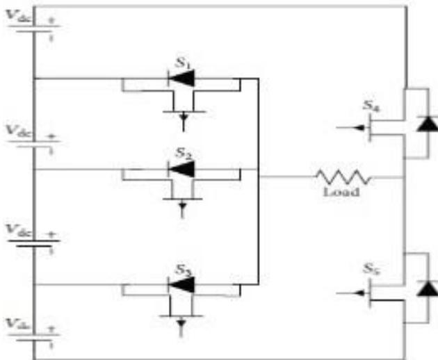
Fig. 1: 5-Switch 7-Level Topology
