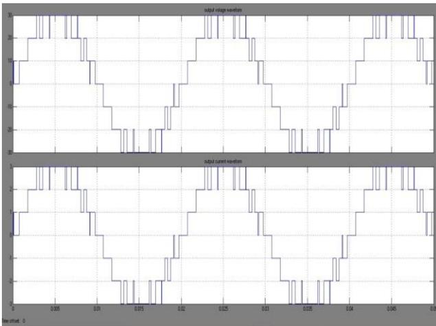
Fig. 4: Output voltage and current waveforms for 7-level MLI
