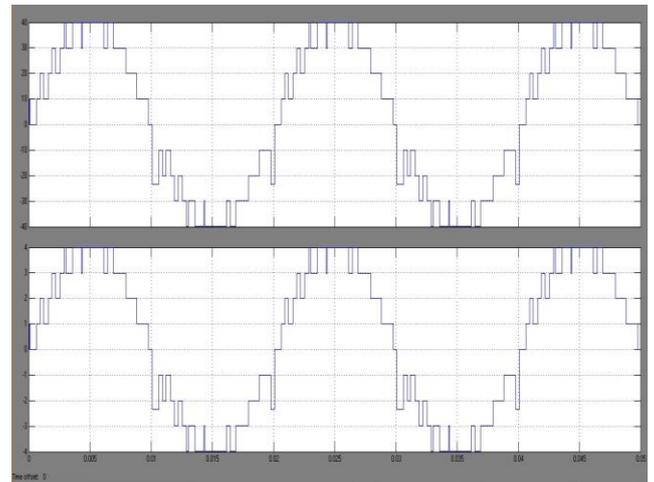
Fig. 13: Output voltage and current waveform for 9-level MLI
