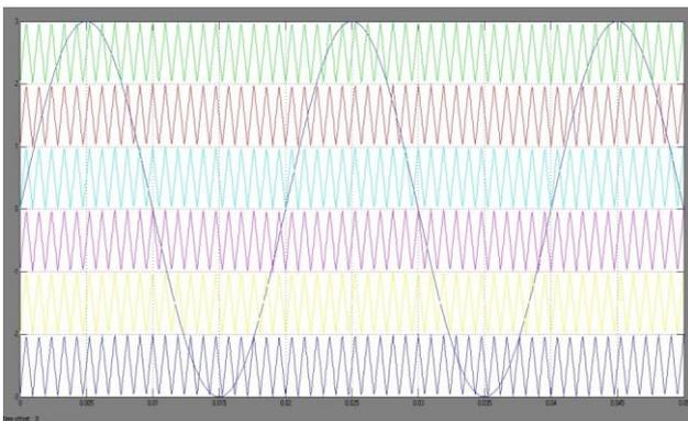
Fig. 5: PD PWM for 7-Level MLI
