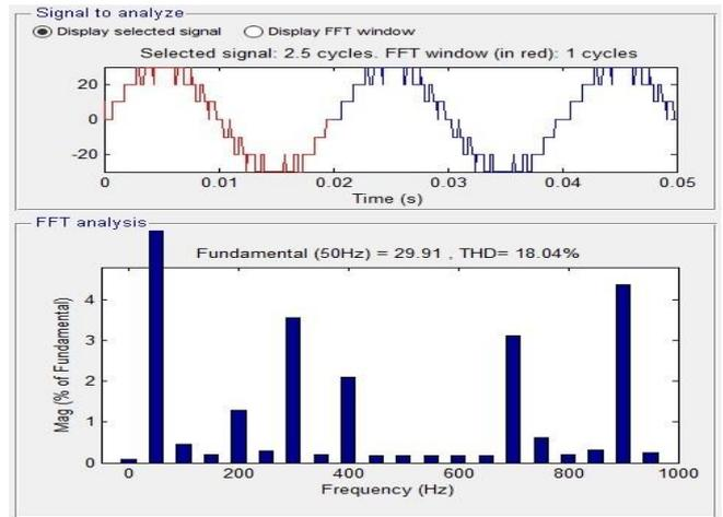
Fig. 9: FFT Analysis for POD PWM of 7-level MLI
