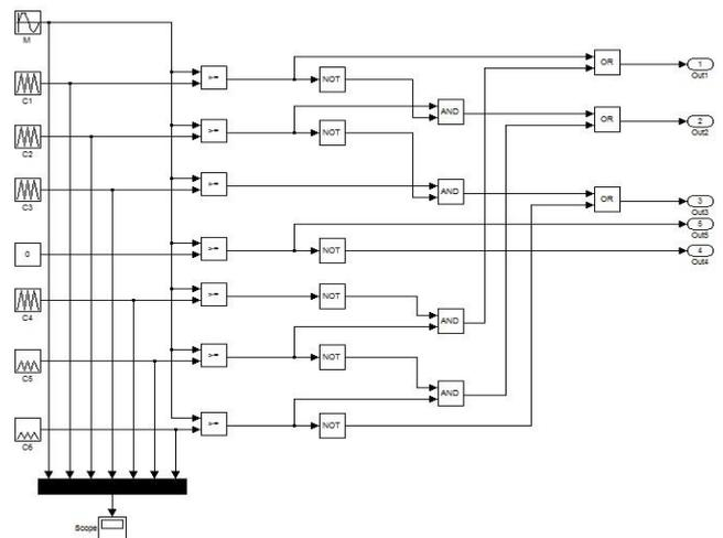
Fig. 3: Sub Circuit for 7-level MLI
