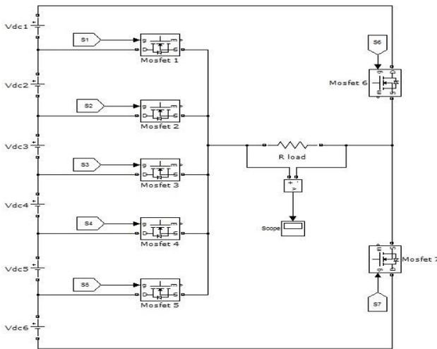
Fig. 17: Simulation circuit for 11-level MLI
