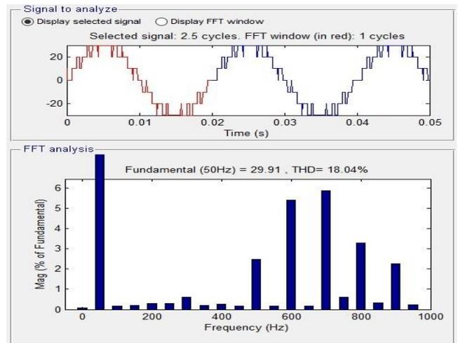
Fig. 10: FFT Analysis for APOD PWM of 7-level MLI
