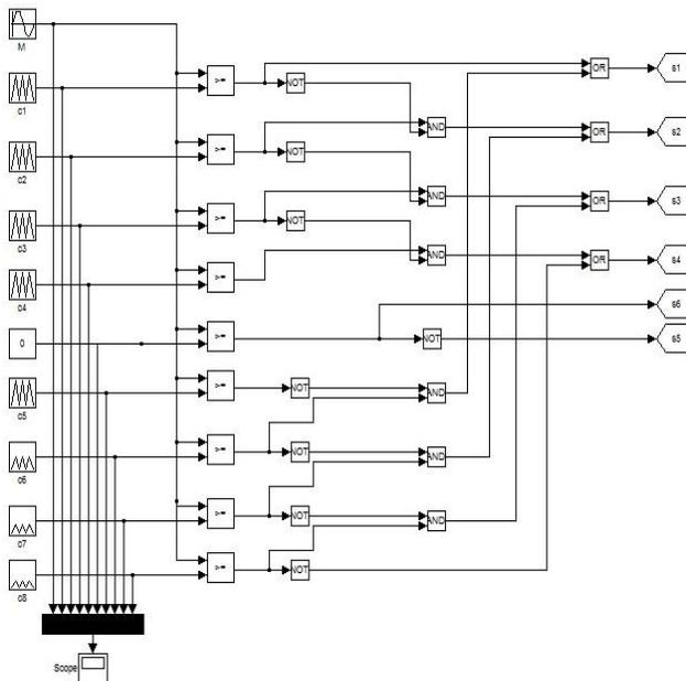
Fig. 12: Sub circuit for 9-level MLI
