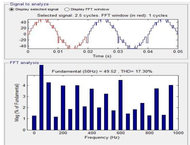
Fig. 22: FFT Analysis for APOD PWM of 11-level MLI
