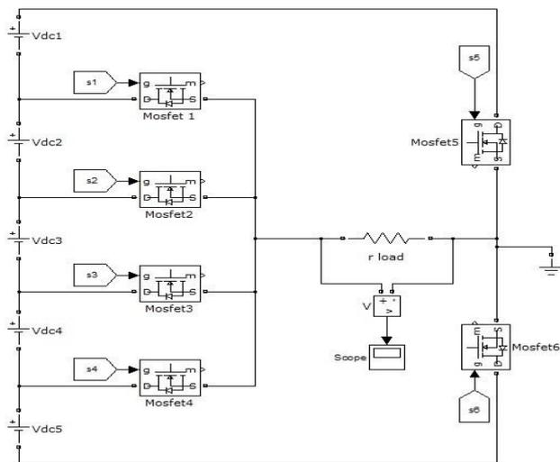
Fig. 11: Simulation Circuit of 6-switch 9-level MLI
