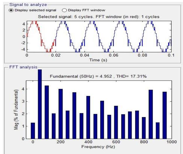
Fig. 20: FFT Analysis for PD PWM of 11-level MLI
