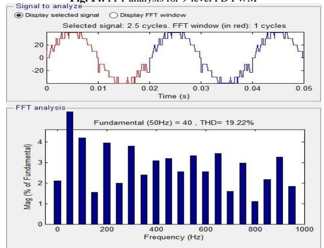
Fig. 15: FFT analysis for 9-level POD PWM
