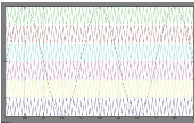
Fig. 7: APOD PWM for 7-level MLI
