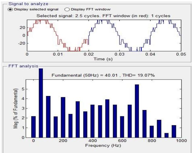
Fig. 16: FFT Analysis for 9-level APOD PWM
