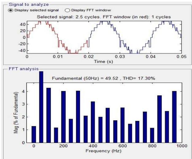
Fig. 21: FFT analysis for POD PWM of 11-level MLI
