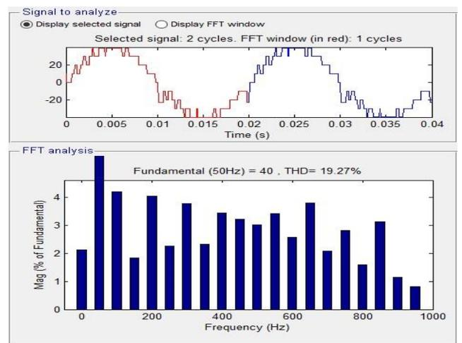
Fig. 14: FFT analysis for 9-level PD PWM
