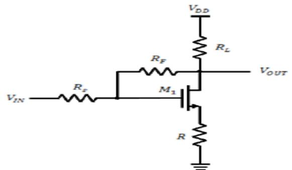
Fig.2(b): Shunt-Series Feedback
