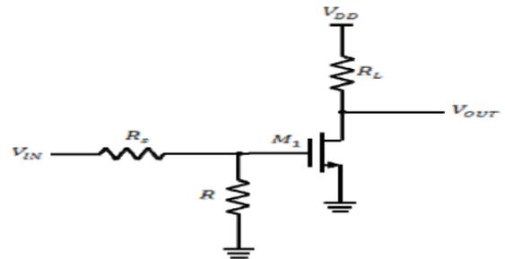
Fig.2(a): Resistive Termination
