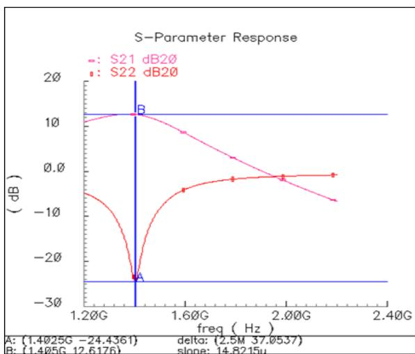
Fig.11: The overall gain of the LNA ( $S_{21}$ ) is 13dB at 1.4025 GHz
