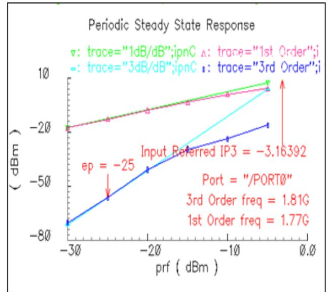
Fig.12: 3<sup>rd</sup> order input intercept point (IIP<sub>3</sub>)
