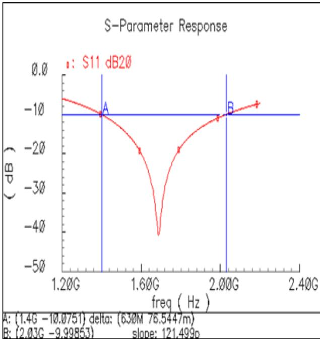
Fig.5: The simulation of input/output return losses.
