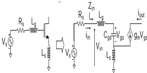
Fig.3: Equivalent circuit of input matching network with source inductive degeneration
