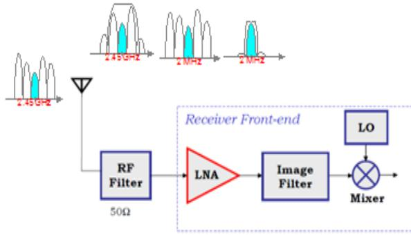
Fig.1: Block diagram of Receiver Font-End
