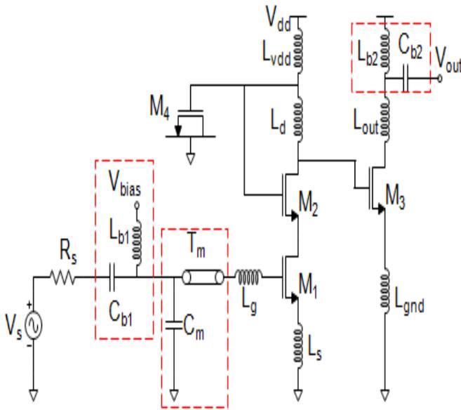
Fig.4: Schematic of proposed LNA
