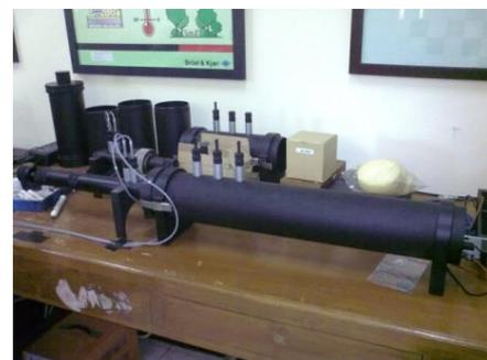
Fig. 11. impedance Tube type 4206 T
