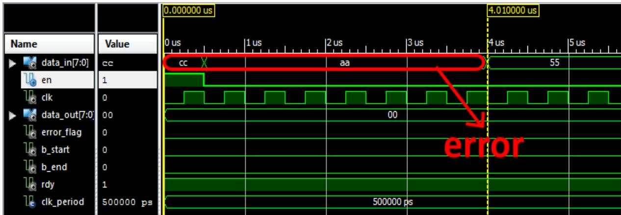
Fig. 13.1: The Decoder Waveform with 8 Bytes Error Showing that Error Occurred Attransmission.
