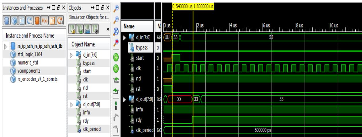
Fig. 11.1: The RS IP Core Waveform Showing Data Flow to and from IP Core Encoder.
