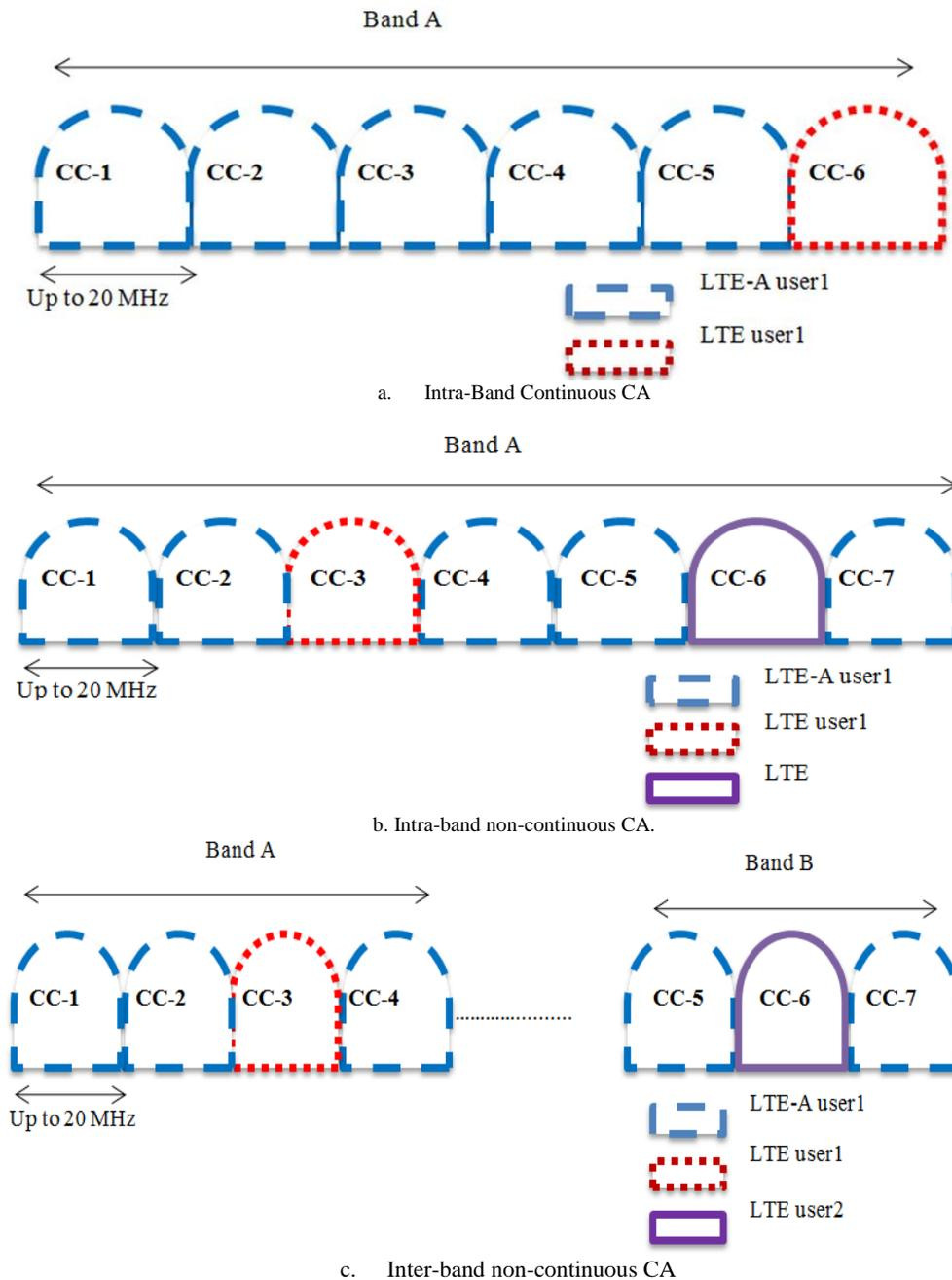
Fig. 11: Types of CA (A) Intra-Band Continuous CA (B) Intra-Band Non-Continuous CA (C) Inter-Band CA [27] Carrier Aggregation Implementation.
