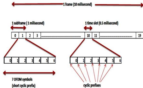
Fig. 8: LTE Generic Frame Structure [24].
