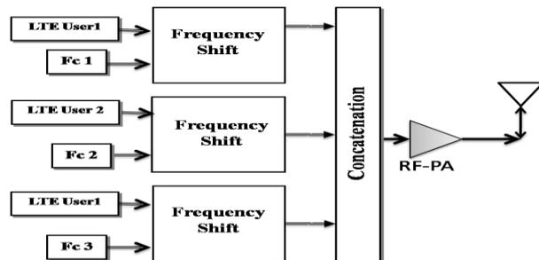
Fig. 13: The Simulink Implemented Block Diagram of Continuous and Non-Continuous Intra-Band CA Downlink Transmitter.
