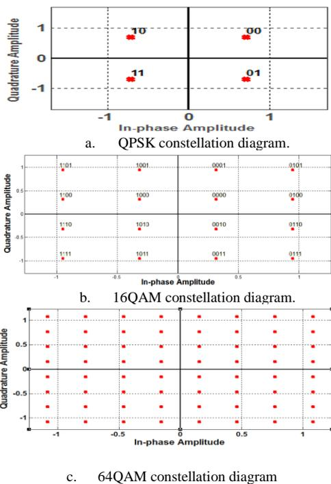
Fig. 4: The Constellation Diagram of Different Mapper Order Used in LTE A. QPSK B. 16-QAM C. 64-QAM
