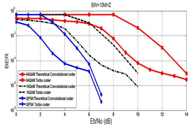
Fig. 15: BER Performance for LTE-A Turbo Coder and Theoretical Convolutional Coder at Different Mapper Order.
