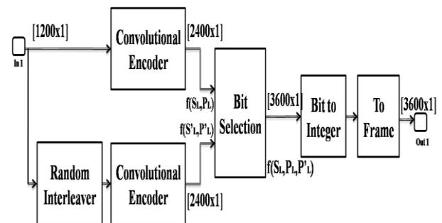
**Fig. 2:** Turbo Encoder Block Diagram.
