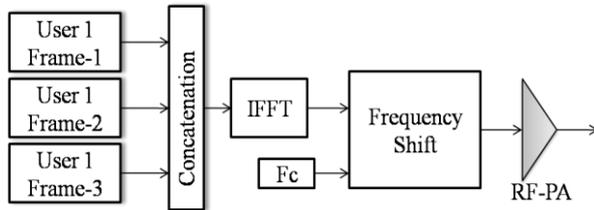
Fig. 12: The Implemented Block Diagram of Downlink Transmitter Continuous CA.
