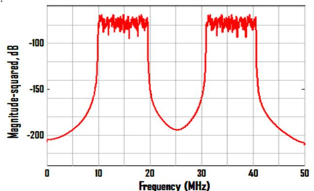
Fig. 16: Two CCs Non-Continuous Symmetric CA 30 MHz
