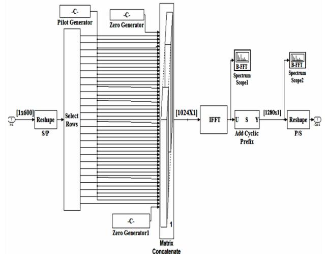
Fig. 5: The Simulink Implemented OFDM Symbol Generator.
