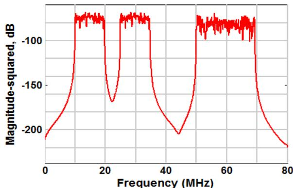
Fig. 18: Three CCs Non-Continuous Asymmetric CA 60 MHz Bandwidth.
