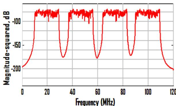
Fig. 19: Non-Continuous Symmetric CA 100 MHz Bandwidth.
