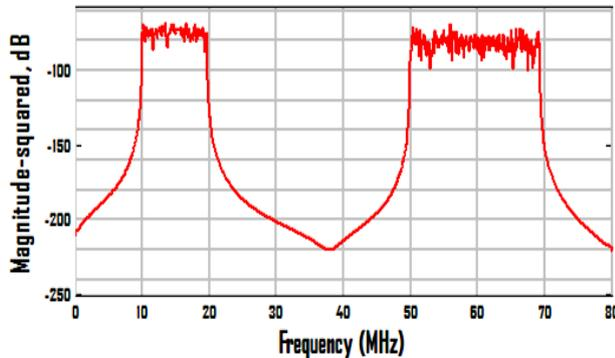
Fig. 17: Two CCs Non-Continuous Asymmetric CA 60 MHz Bandwidth.
