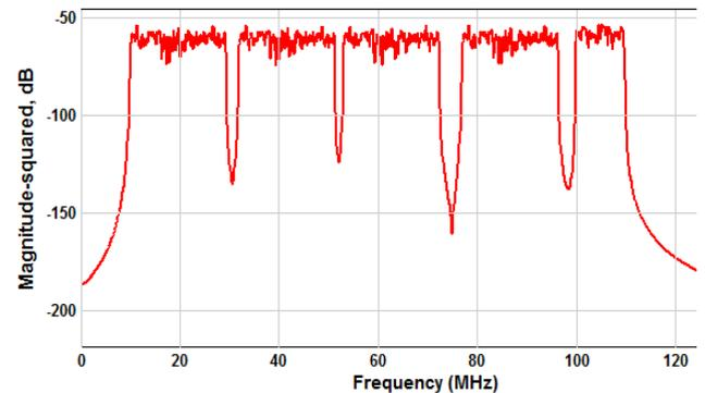
Fig. 20: Non-Continuous Asymmetric CA 100 MHz Bandwidth Using 5 CCs.
