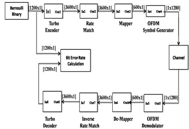
**Fig. 1:** The Basic LTE Downlink Physical Layer Block Diagram using Matlab Simulink
