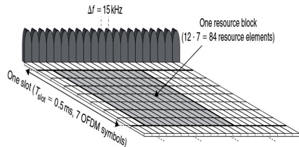
Fig. 9: LTE Downlink Resource Block for Normal Cyclic Prefix [22]
