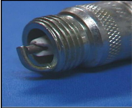
Fig. 6: Photograph of a Broken Starting Tip in the Plug.
