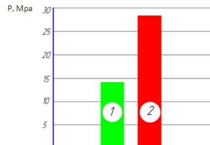
**Fig. 13:** Diagram of the Coupling Oil Retention Force P during Various Treatment Methods. 1 - Reaming Treatment; 2 - Vibro- Rolling Treatment Followed by Broaching Deformation.
