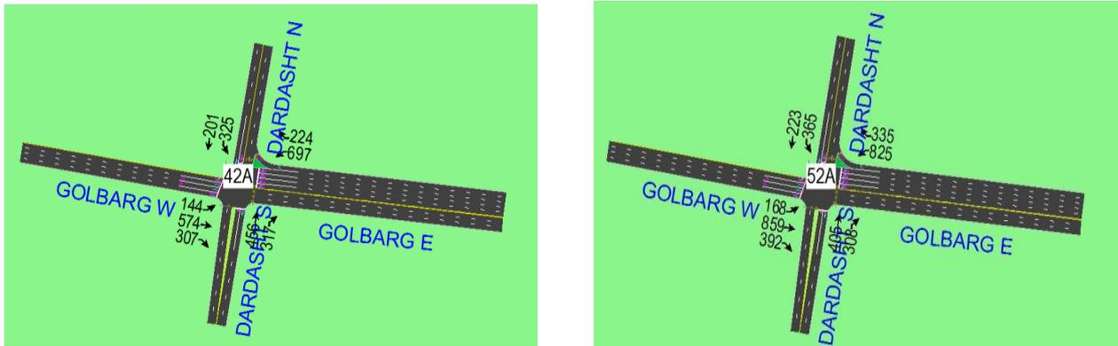
Fig. 5: Cycle Length and Geometric Plan of Golbarg-Dardasht Intersection after Optimization in AM Peak Time by Synchro Software.
