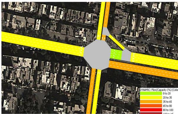
Fig. 7: The Percent of Flow/Capacity in AM Peak Time at Golbarg-Dardasht Intersection.
