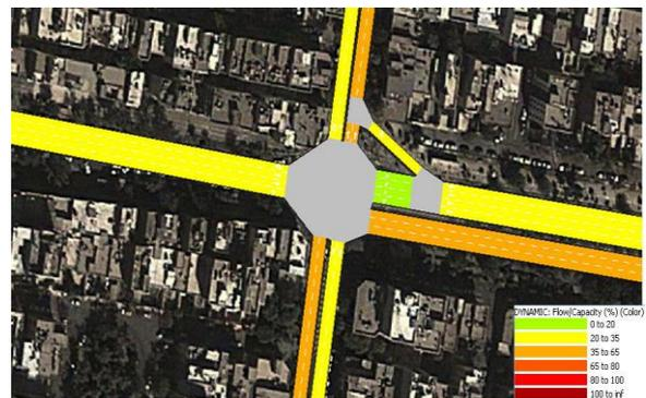
Fig. 4: Percentage of Flow/Capacity, Respectively, During AM and PM Peak Time at Zibadasht-Dehkadeh Intersection
