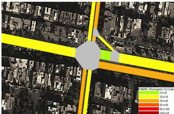
Fig. 3: Percentage of Flow/Capacity, Respectively, During AM and PM Peak Time at Golabar-Dardasht Intersection
