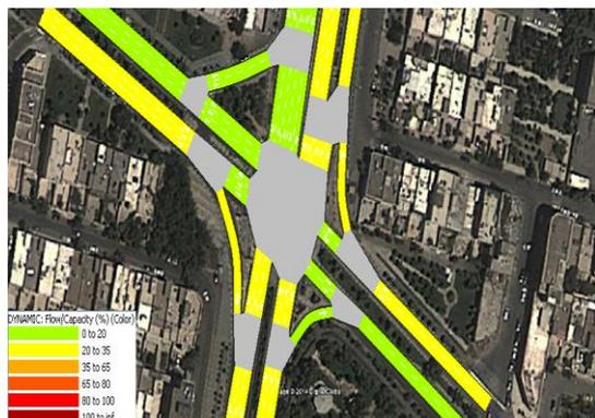
Fig. 8: The Percent of Flow/Capacity in AM Peak Time at Zibadasht-Dehkadeh Intersection.
