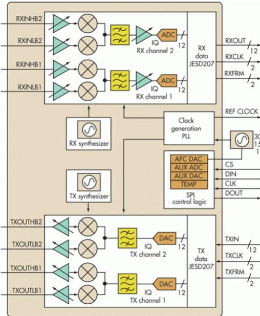
Fig. 2: Maxim Multistandard 3G/4G Transceiver [2].
