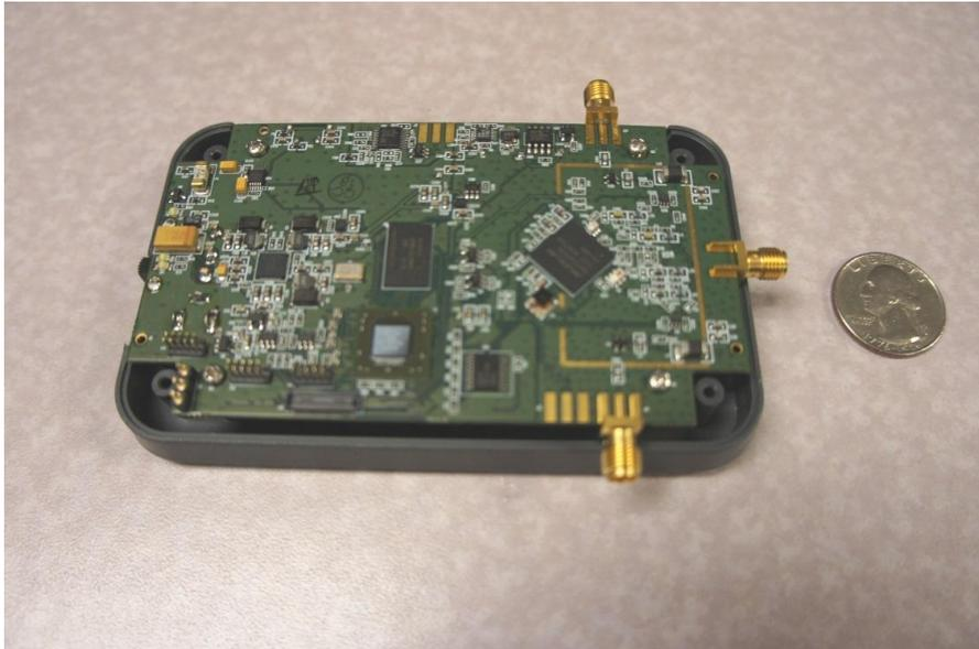
Fig. 4: The OSD SDR Card Top View
