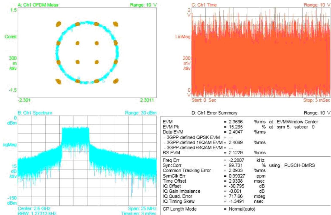
Fig. 7: Snapshot From Agilent MXK N9026A Signal Analyzer
