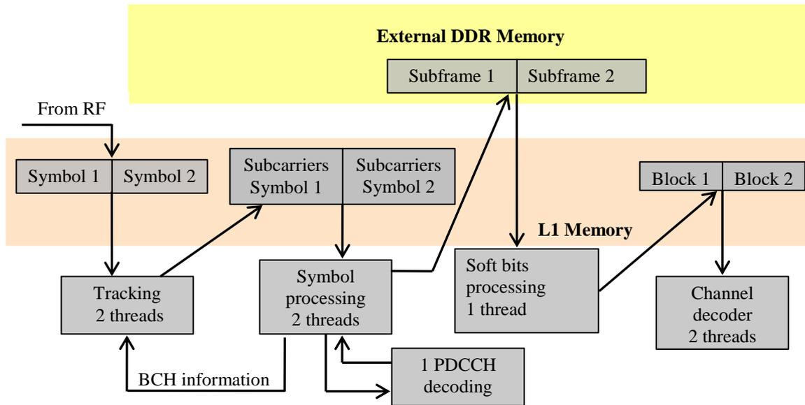
Fig. 5: LTE Partitioning on SB3500
