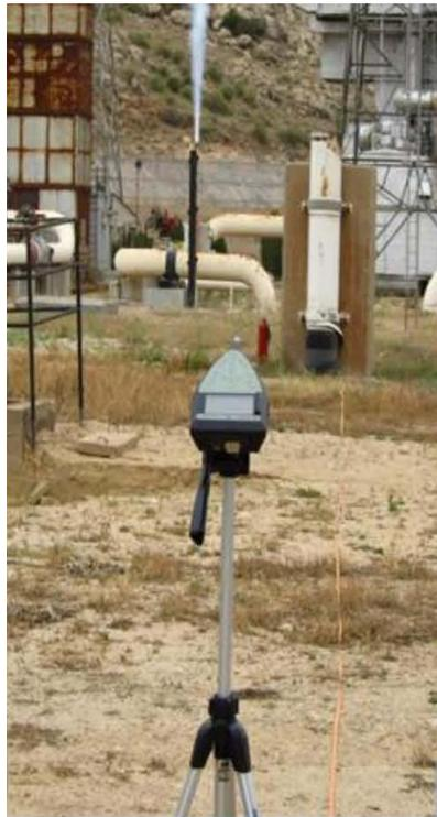
Fig. 1: The Photograph of the Sound Level Meter Used For the Measurements.
