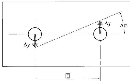
Fig. 4: Maximum Deviation between the Top Surface of the Second Plate and the Bottom Surface of the First Plate around Z-Axis.
