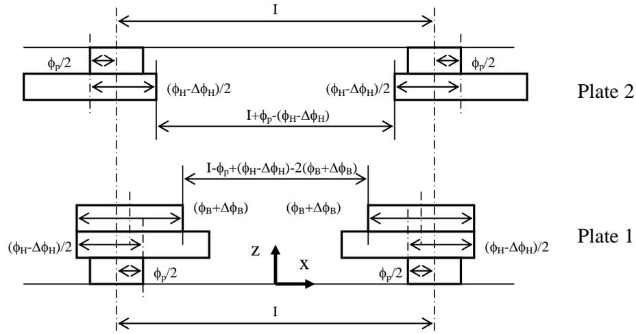
Fig. 5: Assembly Constraint in Worst Case Approach.
