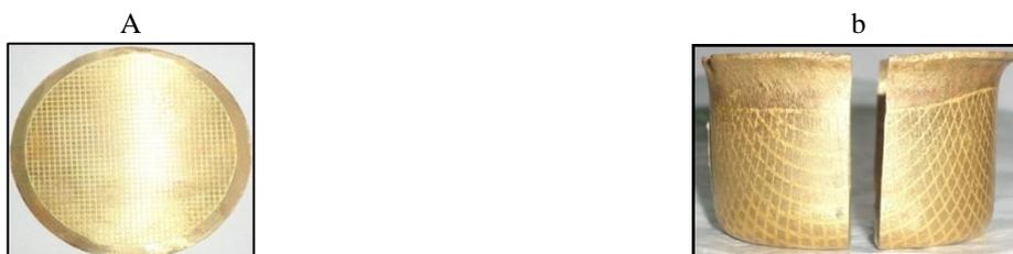
Fig. 6: A) grid square on the blank, B) Sample of forming grid cap
