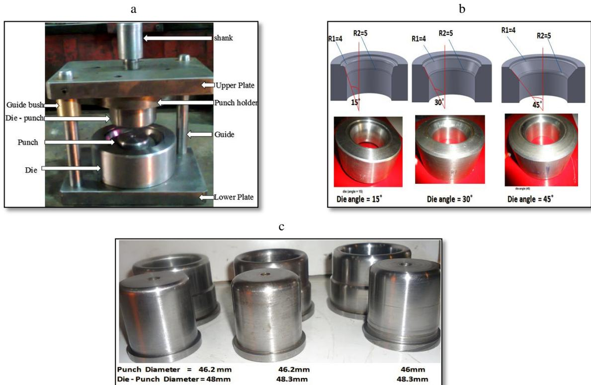
Fig. 4: A) Assembly of Rig B) Dies Geometry C) Punches and(Die-Punches)
