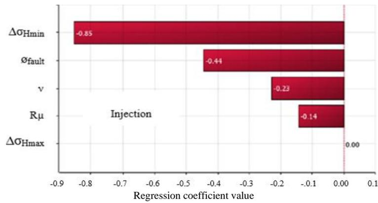
Fig. 7: Critical Pressure Change at the Side burden Parallel to  $\Sigma_{hmax}$  for Injection Scenario.
