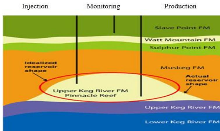
Fig. 6: Geometry of Actual and Idealized Reservoir [19].
