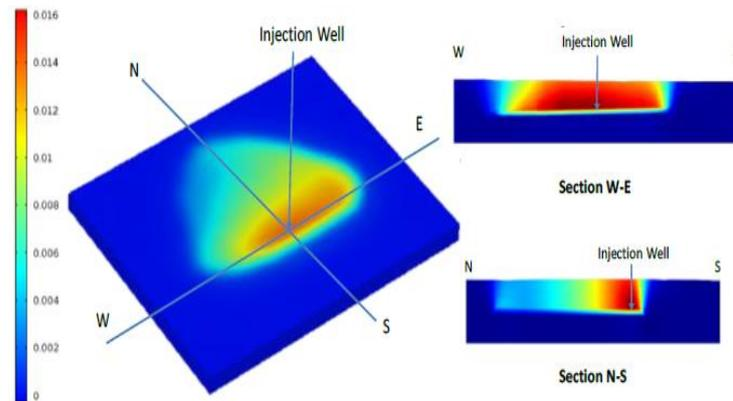
Fig. 4: Distribution of Vertical Deformation after 25 Years of CO<sub>2</sub> Injection.
