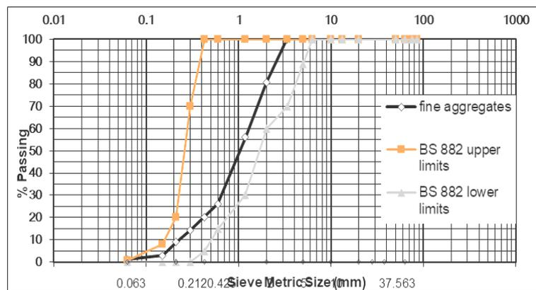
Fig. 1: Particle Size Distribution of the Fine Aggregates.
