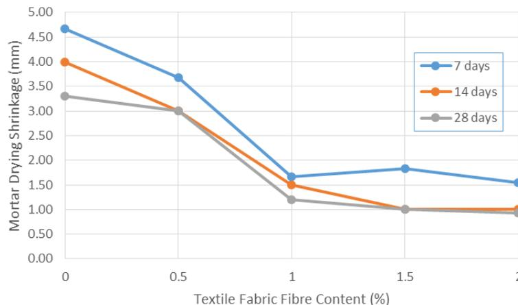
Fig. 6: Effect of Textile Fabric Fibre on Mortar Drying Shrinkage.
