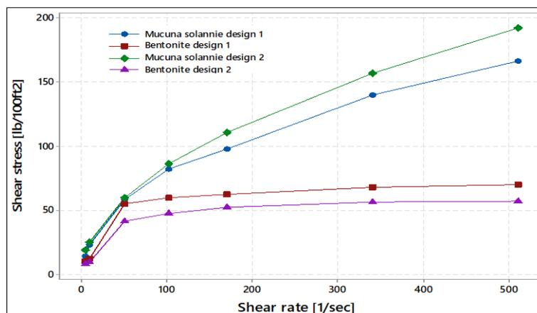
Fig. 6: Mucuna solanmie and Bentonite Rheological Plots At 150°F and 200°F Using Herschel-Bulkley.
