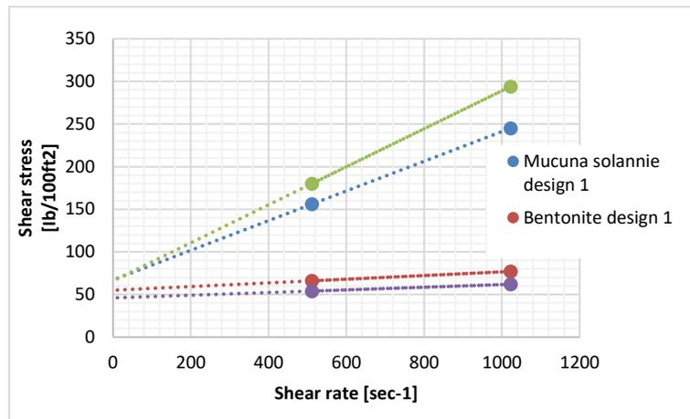
Fig. 5: Mucuna solanmie and Bentonite Rheological Plots at 150°F and 200°F Using Bingham Plastic Model.
