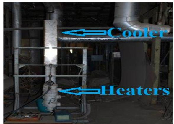
Fig.36: Experiment Setup for Thermosyphon Heat Transfer Device
