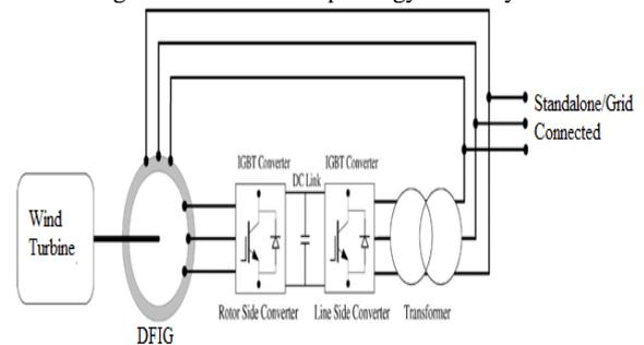
Fig. 1 DFIG connected Wind Turbine
