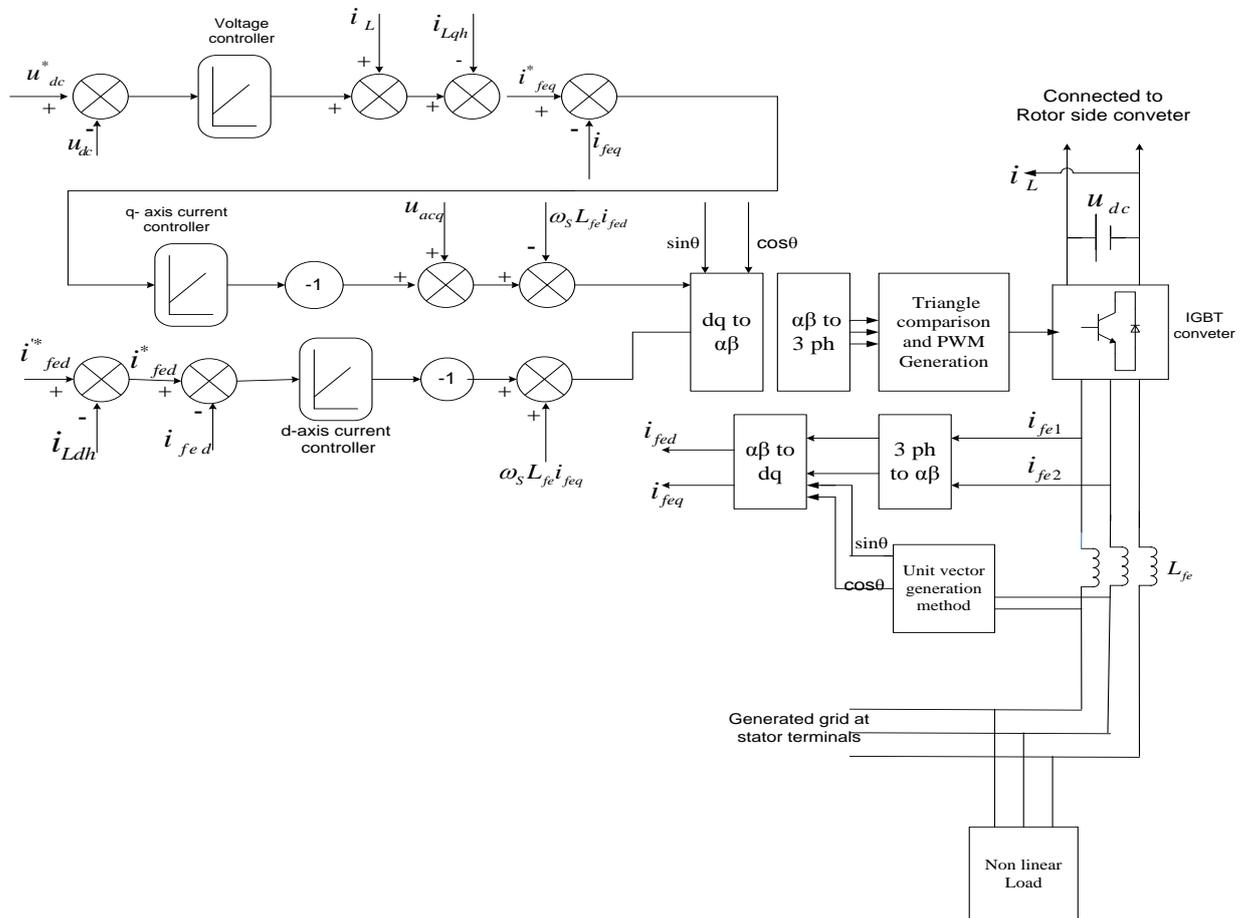
**Fig. 8** Block diagram of line side converter
