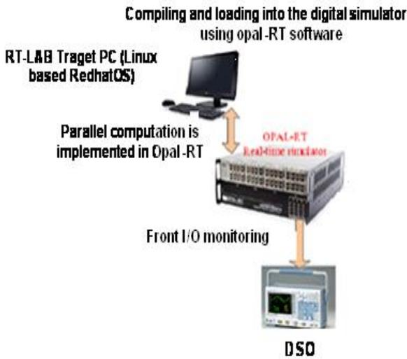
Fig. 10. Opal-RT and RT-Lab Architecture
