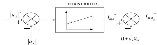
Fig. 3 configuration of voltage control loop
