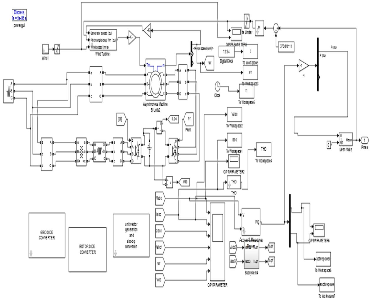
FIG. 9 Simulation model of DFIG with back to back PWM converter
