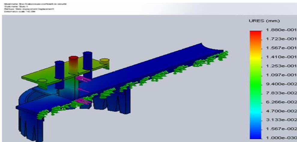
Fig. 9: Displacements Distribution on the Breaking Arm of the Cocoa Pod.
