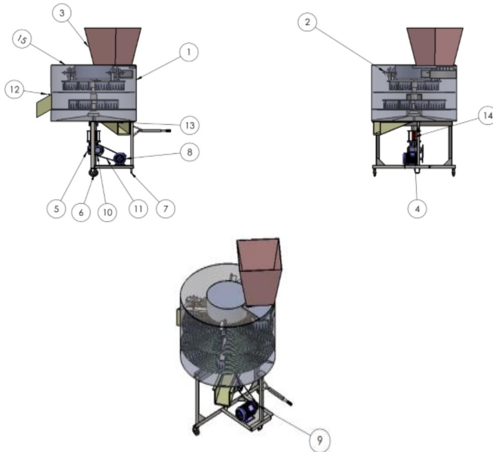
Fig. 10: The Cocoa Pod Breaking and Extraction Machine.
