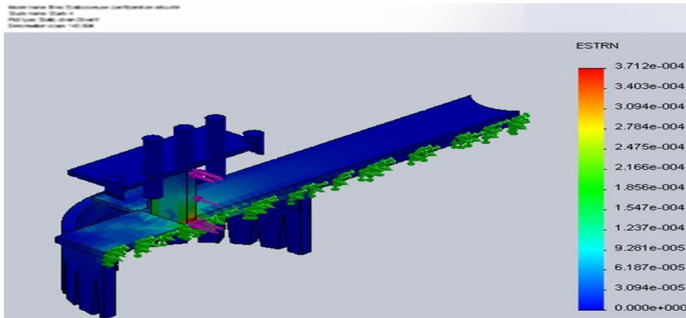
Fig. 8: Strains Distribution on the Breaking Arm of the Cocoa Pod.
