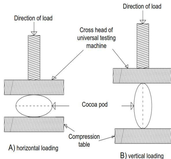
Fig. 4: Orientations of Cocoa Pod During Quasi-Static Compression Tests.
