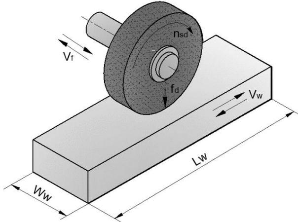
Fig. 1: Schema of Surface Grinding.
