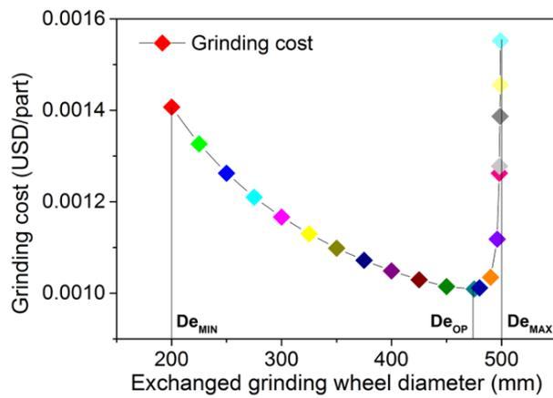
Fig. 2: Grinding Cost Versus Exchanged Grinding Wheel Diameter.
