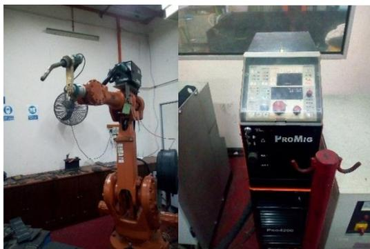
**Fig 1:** ABB IRB 2400/16 Robotic welding Machine (left) and KEMMPI ProMig 540 MXE (right)
