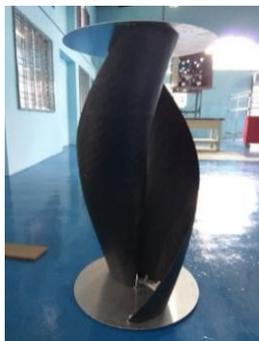
**Fig. 2:** Savonius rotor with 180-degree twist angle model fabricated using 3D printer.
