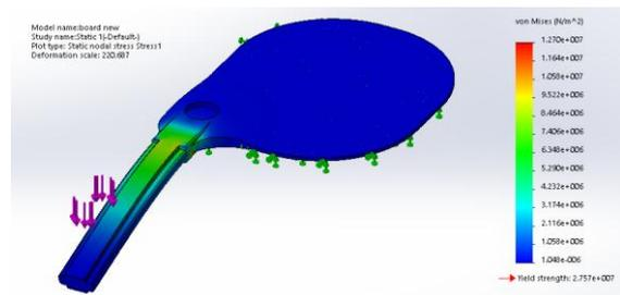
Figure 9: von Mises stress of the board.
