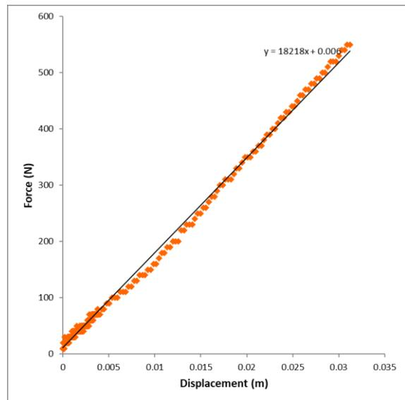
Fig. 4: Suspension stiffness coefficient testing result
