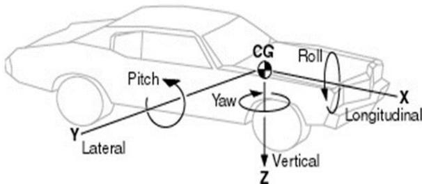
Fig. 1: Vehicle coordinate system
