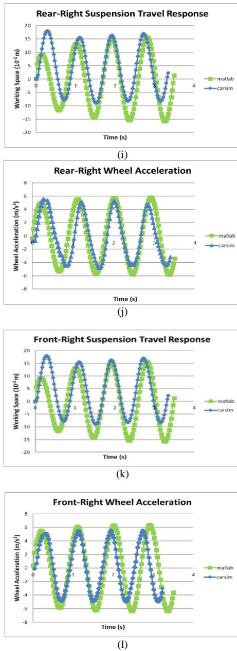
**Fig 5:** Validation graphic of: (a) body displacement response, (b) body acceleration response, (c) pitch angle response, (d) roll angle response, (e) front-left suspension travel response, (f) front-left wheel acceleration response, (g) rear-left suspension travel response, (h) rear-left wheel acceleration response, (i) rear-right suspension travel response, (j) rear-right wheel acceleration response, (k) front-right suspension travel response, and (l) front-right wheel acceleration response.
