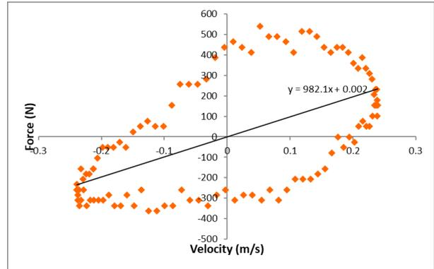
Fig. 3: Suspension damping coefficient testing result
