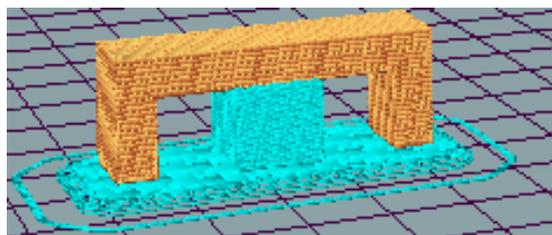
(a) Prototyping direction 0°, Sample No. 1
