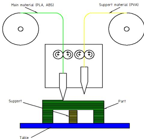
Figure 1: The principle of FDM device with two extrusion heads
