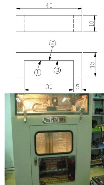
(a) Experimented samples (b) FDM device with two extruders
