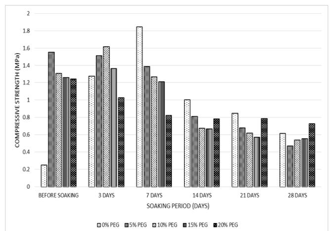
**Figure 8:** Compressive strength of CPC/PEG with the P/L ratio of 1.7 after soaking in Ringer's solution for 28 days.
