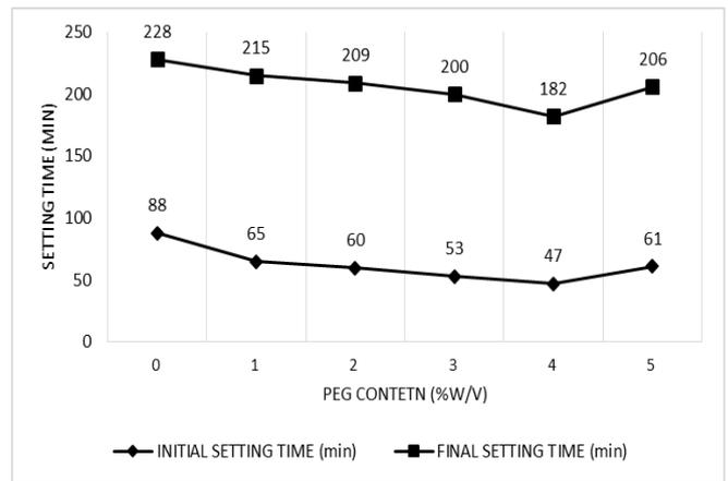
Figure 1: Effect of PEG addition on setting times of CPC prepared with the P/L ratio of 1.3.
