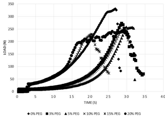
**Figure 4:** Effect of PEG addition on injectability of CPC prepared with the P/L ratio of 1.7.
