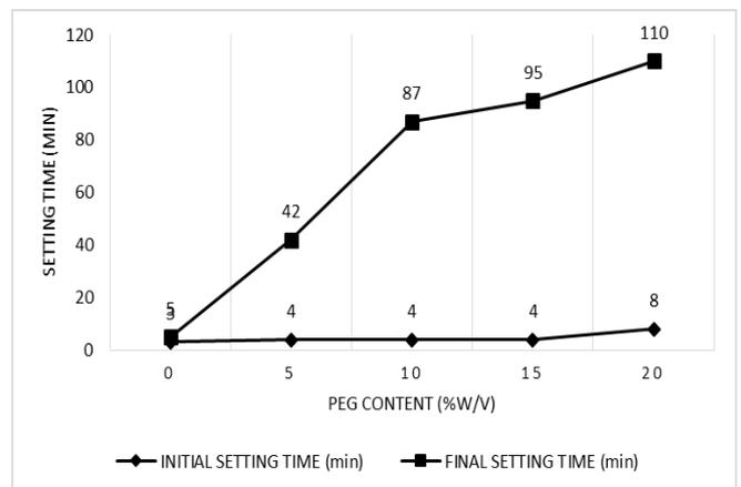
Figure 2: Effect of PEG addition on setting times of CPC prepared with the P/L ratio of 1.7.
