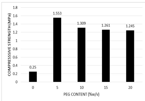
**Figure 6:** Effect of PEG addition on the compressive strength of CPC prepared with the P/L ratio of 1.7.
