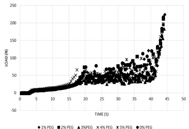
Figure 3: Effect of PEG addition on injectability of CPC prepared with the P/L ratio of 1.3.
