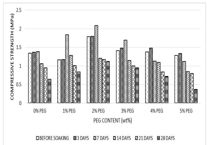
**Figure 7:** Compressive strength of CPC/PEG with the P/L ratio of 1.3 after soaking in Ringer's solution for 28 days.
