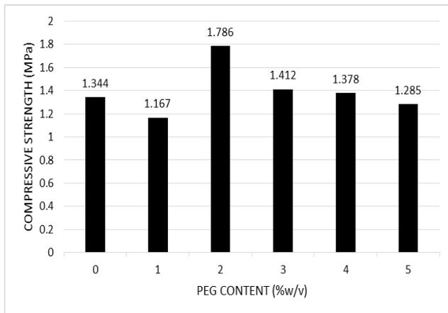
**Figure 5:** Effect of PEG addition on the compressive strength of CPC prepared with the P/L ratio of 1.3.
