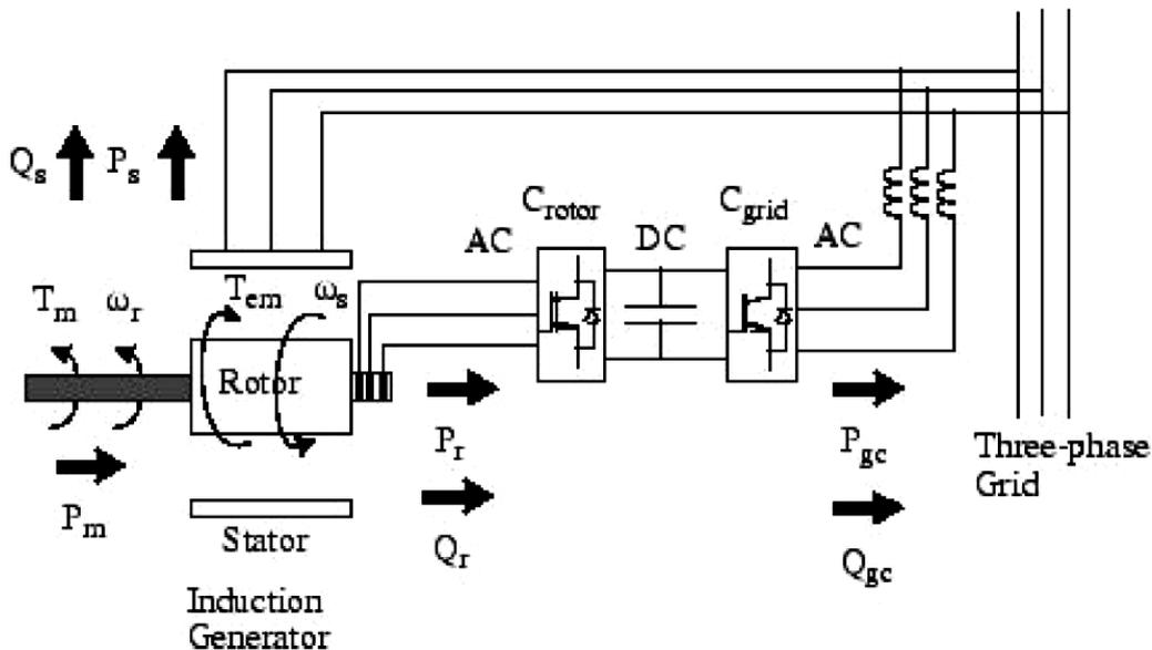
Figure 2: The flow of power on a Doubly Fed Induction Generator (DFIG)
