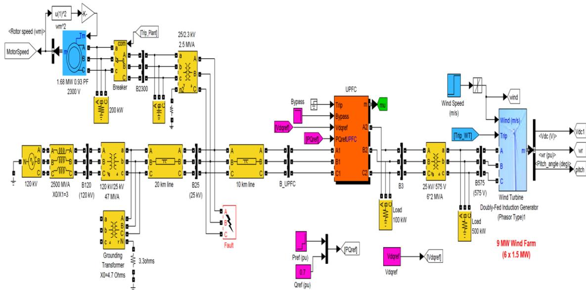
Figure 3: Test system model diagram
