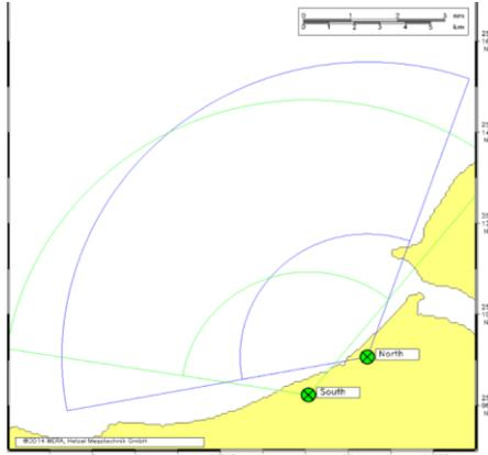
Figure 2: Range and position of radar systems used for the case study in Taipei.
