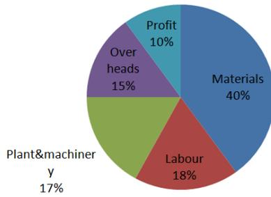
Fig. 5: Distribution of cost elements for cast-in-situ construction (in %)
