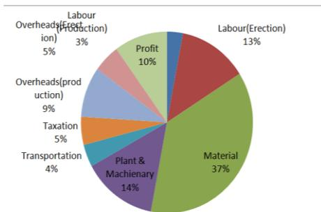
Fig. 6: Distribution of cost elements for Pre cast construction (in %)
