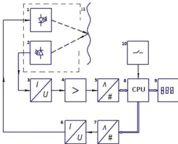
**Fig.1:** Functional diagram of the device for the optical study of the structure of biological tissues.
