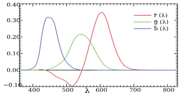
**Fig.2:** RGB spectrum of the visible range
