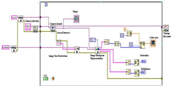
**Fig.3:** Functional diagram of the device implemented in the LabView environment
