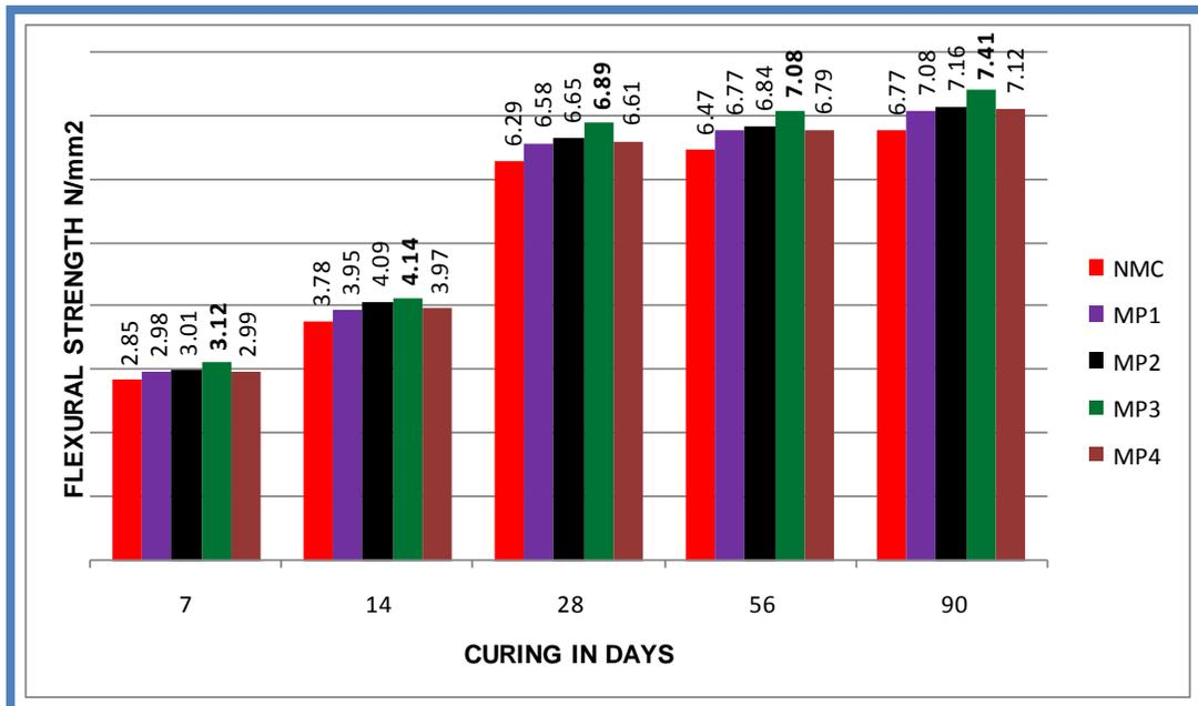
Fig.6: Comparison of Flexural Strength Test Results (Bending stress Vs curing in days)
