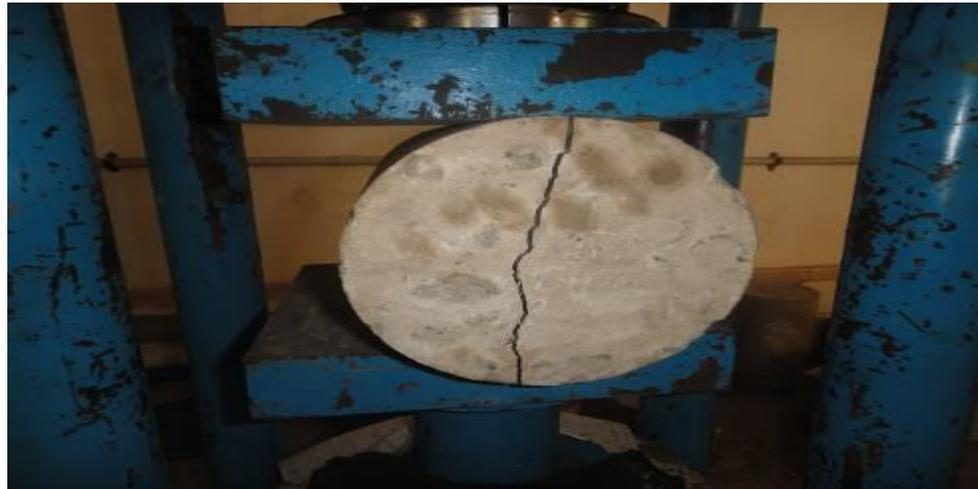
**Fig.3:** Split Tensile Strength Test
