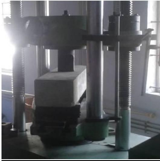
Fig.5: Flexural Strength Test
