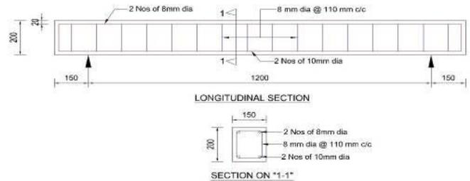
Fig.7: Reinforcement details of RC flexural beam
