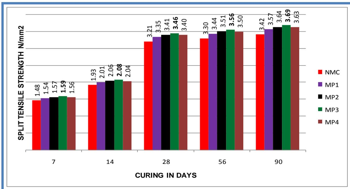
**Fig.4:** Comparison of Split Tensile Strength Test Results
