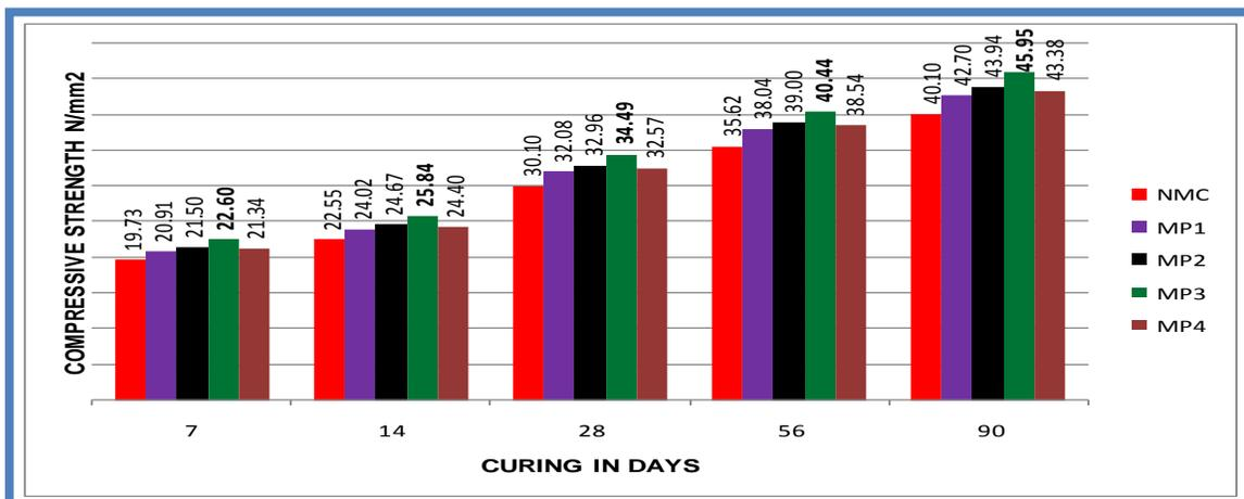
**Fig.2:** Comparison of Compressive Strength Test Results
