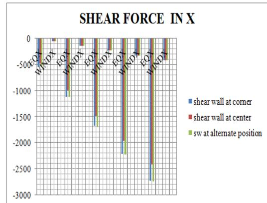
Fig.6 Shear Force in X
