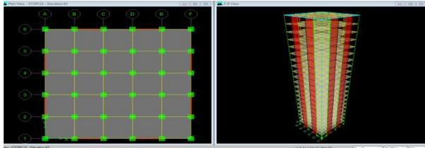
Fig.3 Shear wall at alternative positions
