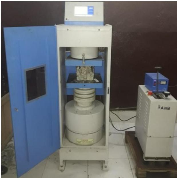
Figure 11 Split Tensile Testing Machine
