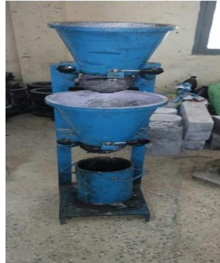
Figure 2 Compaction factor test on concrete
