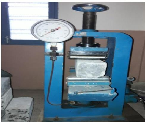
Figure 7 Flexural strength testing machine
