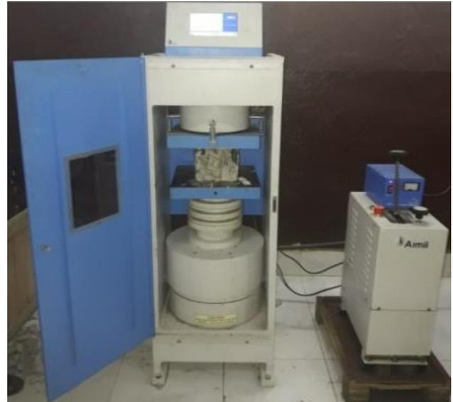
Figure 4 Compression Testing Machine
