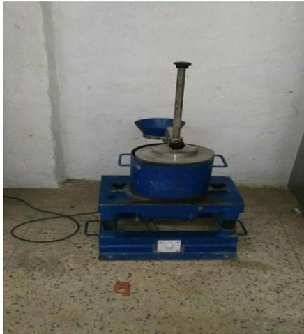
Figure 3 Vee Bee Consistometer
