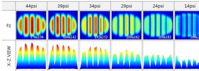
Fig. 7: Tire Contact Pressure Distribution by Tire Air Pressure.
