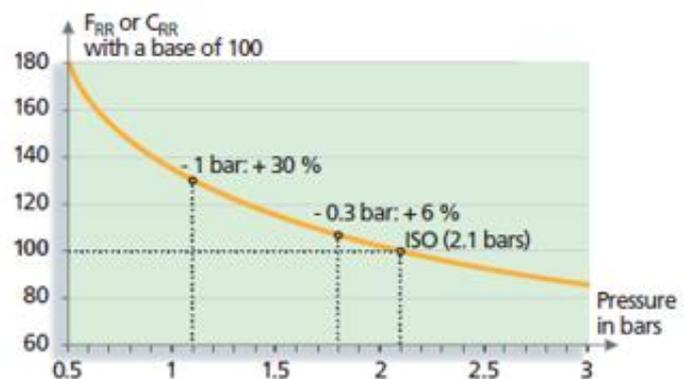
Fig. 6: Effect of Tire Air Pressure (Passenger Car) [5].
