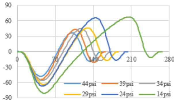
Fig. 8: The Characteristics of Force X by Tire Air Pressure.
