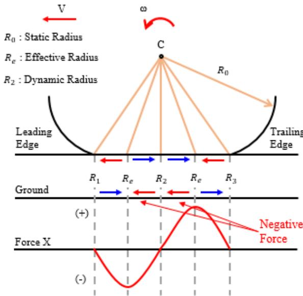
Fig. 4: Rolling Resistance Mechanism.
