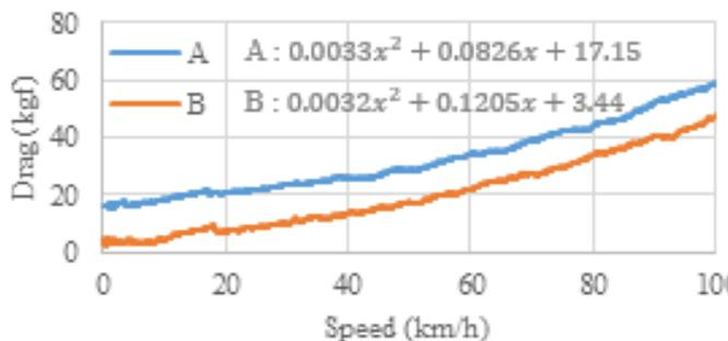
Fig. 9: The Comparison of the Running Resistance.
