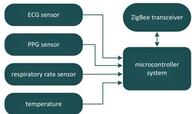
**Fig. 2:** The block diagram of Sensor Device.
