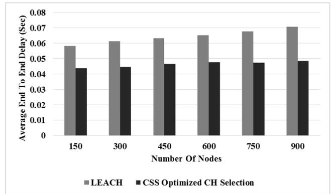
**Fig 2:** Average End to End Delay for CSS Optimized CH Selection
