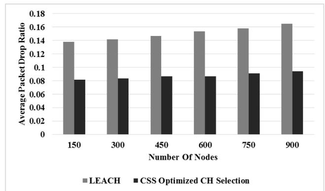
**Fig 3:** Average Packet Drop Ratio for CSS Optimized CH Selection
