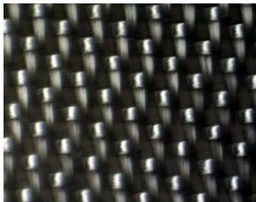
**Fig. 10:** Simple Texture S-2 Glass with Direct Strings (57×57 for Each Inch) Used to Make Fiber-Metal Multilayers.
