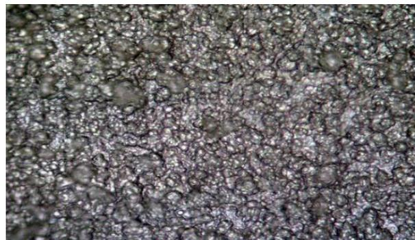
Fig. 4: Aluminum Oxide Layer Obtained From PAA with 40x Magnification.
