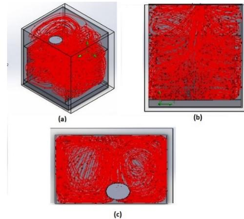
Fig. 11: (A) Flow Viewed in 3D, (B) Flow Viewed from Front and (C) Flow Viewed from Top.
