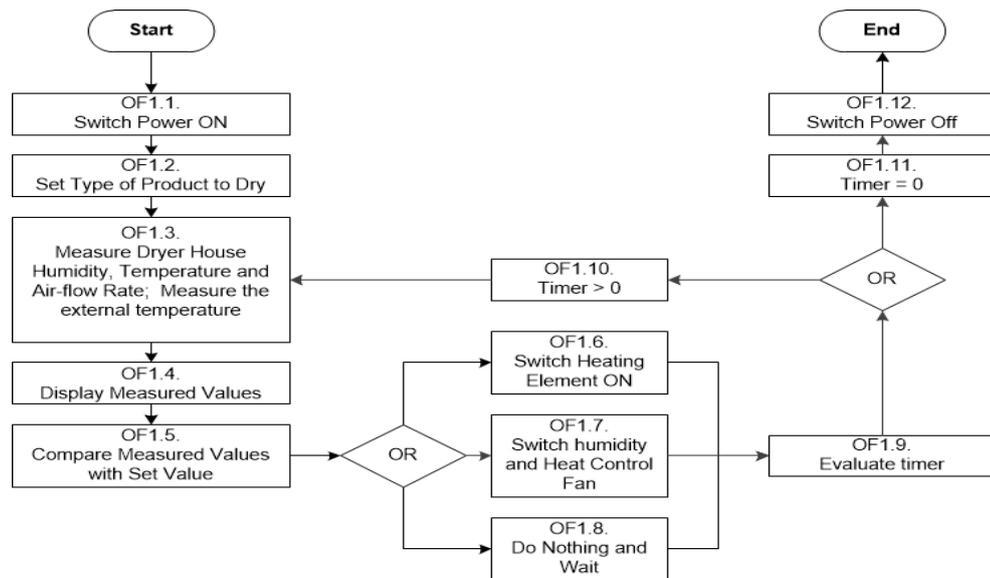
Fig. 2: System Operational Flow
