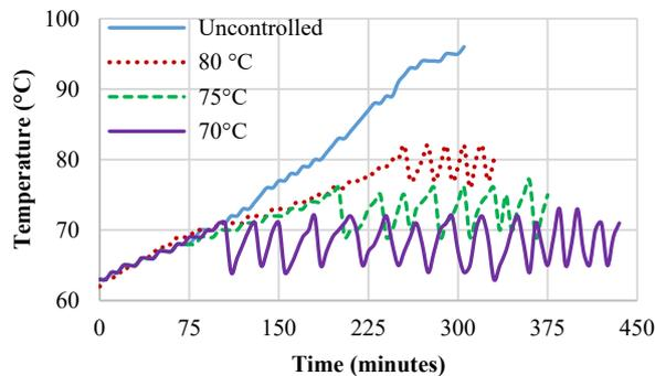
Fig. 15: No Humidity Extraction Fan Temperature Profile.
