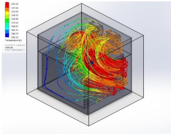
Fig. 7: Simulations with All Fans Active.
