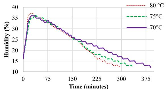
Fig. 18: Humidity Profile with the Extraction Fan Included.
