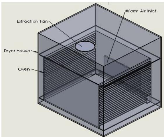
Fig. 9: Single Top Humidity Extraction Fan Assembly.
